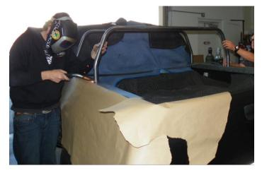
Place Front hoop ½" from front edge of bed rail, centered from side to side and tack weld in place. Be careful welding on top of plastic bed rails, they will melt with too much heat. Place center hoop on center line from earlier, centered left to right and tack weld in place. Place rear hoop ½" from rear of bed rail and tack in place.
