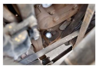
**STEP 2**Remove dipstick bracket hardware.
