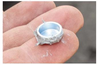
**STEP 6**Lightly tap freeze plug to secure it into place.
