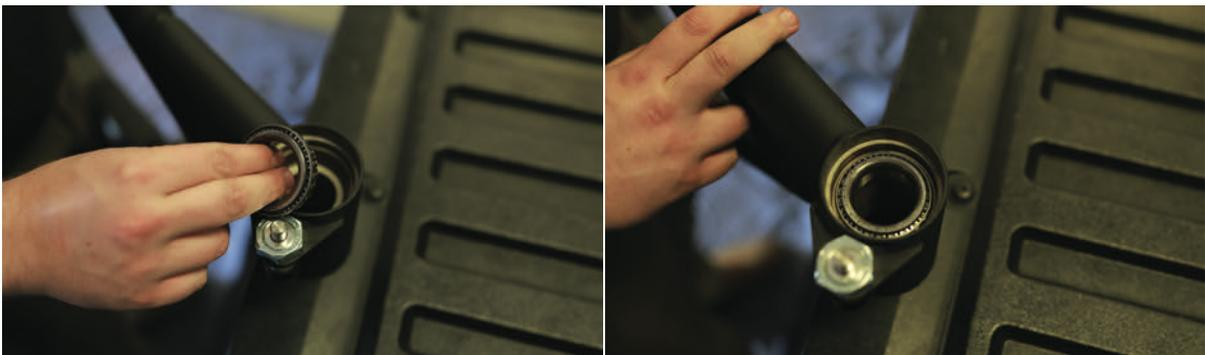
Add a small amount of grease around the lower edge of bearing housing cap for ease of installation and better sealing.
