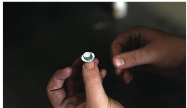
Using the  $\frac{3}{4}$ " long  $\frac{1}{4}$ -20 screws and  $\frac{1}{4}$ " washers to install the license plate on the flip up bracket.
