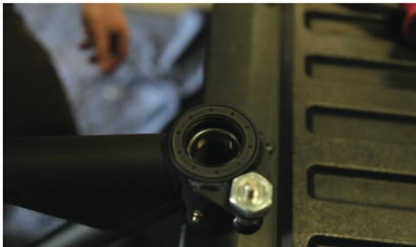
Continue tapping the seal in until it is flush with the housing as shown above. After the seal is installed lightly grease the seal lips.
