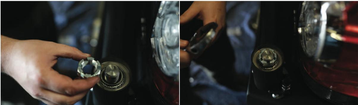
Fasten the castle nut onto the top of the spindle as shown above.
