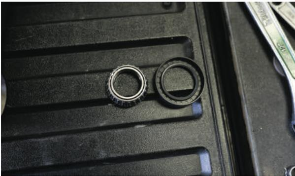
To install the tire carrier arm, begin with the larger tapered roller bearing and the rubberized grease seal.
