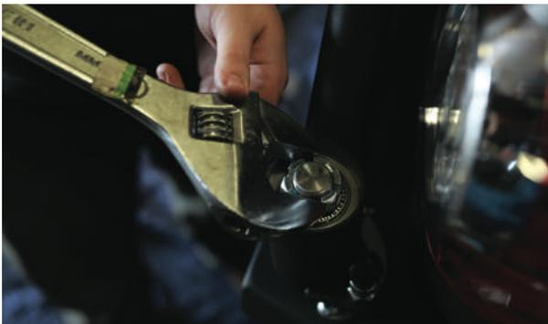
When tightening be sure to align one set of slots in the castle nut with the pin hole on the spindle.
