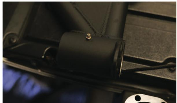
Install the provided Zerk grease fitting on bearing housing as shown. Torque to 15ft-lbs.
