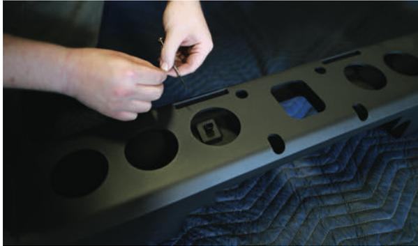
Flip the bumper over and use a small screwdriver as shown to install the small mounting screws. .
