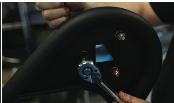
Add the washers and nuts to the back side of the swing arm. Torque the fasteners to 120ft-lbs.
