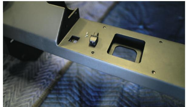
Remove the backup camera from the tailgate and save the 2 small screws that mounted it in place.
