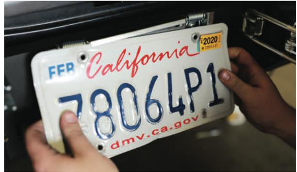
Slide the license plate into the top notch of the bracket, then align the bottom holes with the bolts sticking out of the flip up bracket.
