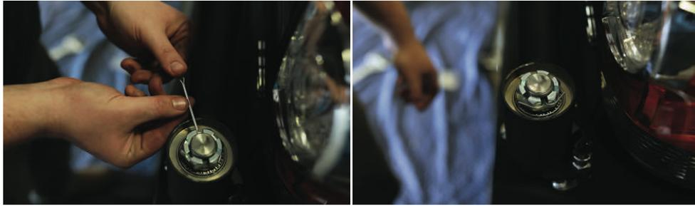
Inset the cotter pin through the castle nut and the spindle hole. Once the cotter pin is fully inserted, bend the legs around the castle nut as shown.
