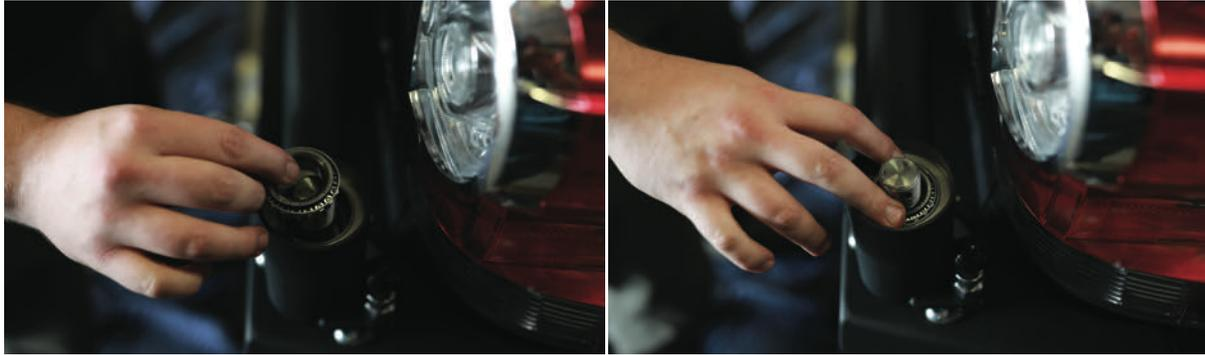
Grease the smaller taper roller bearing, gently insert it into the housing. You may have to lift the swing arm in order to seat the bearing fully.
