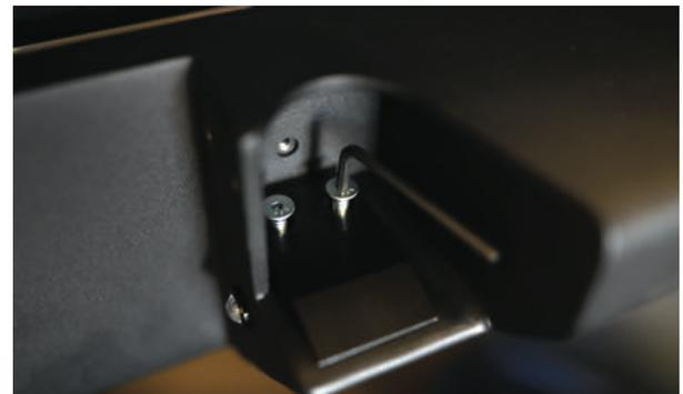
Using a 5/32 hex key, tighten the flat head cap screws down as far as possible.
