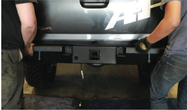
Be sure to save the 6 mounting bolts from the stock bumper. With the help of a friend begin to lift the bumper into position. If you have installed the high clearance hitch you can rest the bumper on it and make small adjustments to align the bumper's mounting holes as needed. If you don't have the hitch you may want a 3rd or 4th person underneath the truck to insert the bolts while it is being held in place by the first two people.
