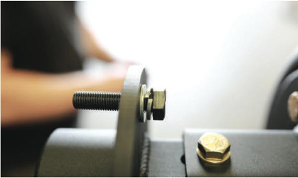
Install the black bolts, lock washers, and flat washers as shown above on all three threaded holes. Torque the bolts to 120ft-lbs.
