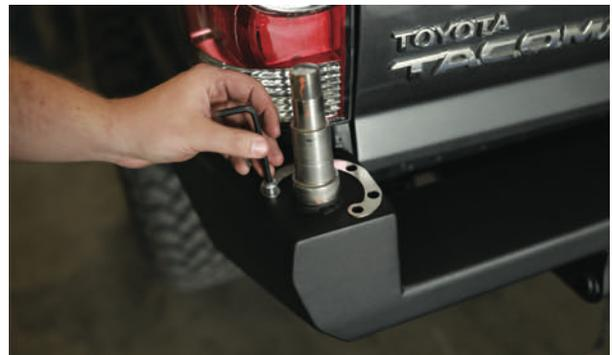
Install the wear plate as shown on the bumper using provided 3/8"-16 button head cap screws.
