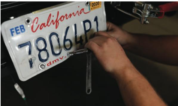
Using another 1/4" flat washer and provided 1/4-20 top lock nut, tighten the bolts that hold the license plate.
