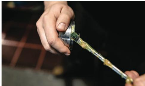
Add a small amount of grease around the lower edge of bearing housing cap for ease of installation and better sealing.
