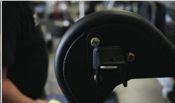
Begin to add the bolts to the bracket and place it on the tire carrier swing arm.
