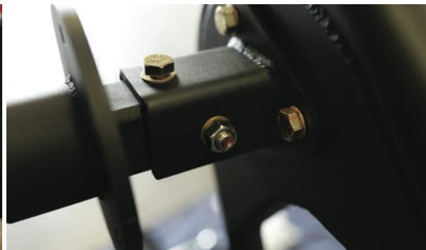
Insert the longer bolt through the side of the base bracket as shown above and secure with washer and nut on opposite side. Torque these bolts to 120ft-lbs.
