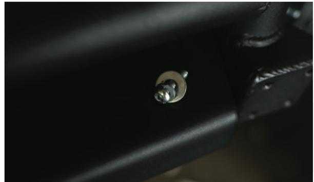
Be sure to put the lock washer between the bolt and the flat washer.
