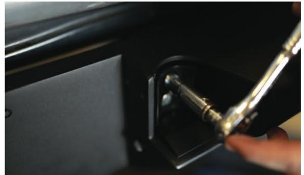
Tighten down both bolts to 12ft-lbs of torque.
