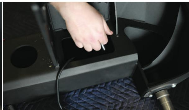
Tighten screws and nuts with provided hex wrench and a deep well socket. Repeat this process for the opposite side of bumper.
