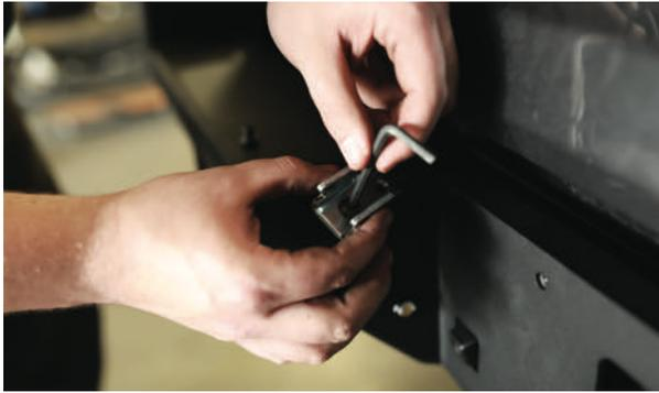
Starting with the hole shown above, use a hex key to install the anchor bracket on the bumper.
