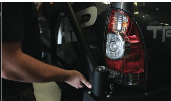
Gently begin to place the swing arm on the spindle. The bearing is seated properly when the arm is able to move down as far as depicted above.
