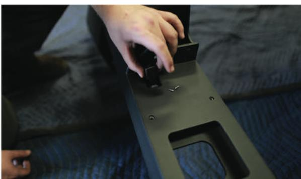
Insert the camera into the mounting bracket as shown. **Note:** it will only insert one way and it may be a tight fit.
