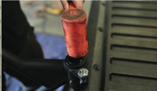
Place the grease seal as shown on the bearing housing and begin to tap it in with a hammer.
