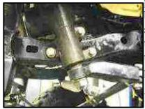
points should from a flat plane for the box to mount to. Only a small weld will be possible on the outside of the sleeve. The remainders of the two sleeves stick out on the inside of the frame. Here you can get a good weld, but don't turn the welder up too high as the back side of the frame is a little thinner than the rest of it. Next take the bracket that welds on top of the frame put in position for the top mount.
