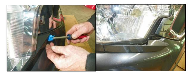
Remove the 6 screws. Using a clip remover, remove the 7 clips.
