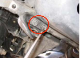
**3.)** Remove lower bumper fascia screws and clips from the driver and passenger side frame rails using a #2 Phillips screw driver.
