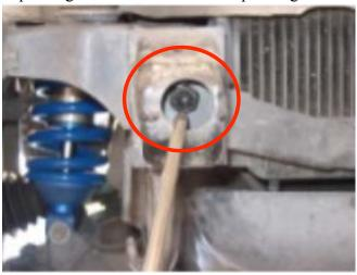
**7.)** Remove factory skid plate from truck using 10mm-14mm sockets. There are seven total fasteners for the stock skid.
