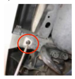
**4.)** Remove driver and passenger side outer bumper mounts using a 14mm socket.
