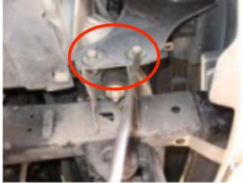
**5.)** Remove driver and passenger side bumper rear mounts using a 12mm socket. To reach these bolts, work the socket through the inner fender wheel well splash guard access hole. Make sure someone is helping with removal or stock bumper is supported during this process as it will be free once these bolts are removed from either side.
