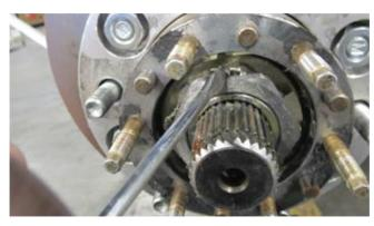
**STEP 6**Remove spindle nut, and star washer
