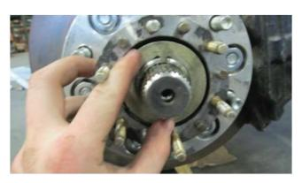
**STEP 10**Install TG spindle washer
