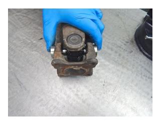
Slide the spider to the mid point between the two cap. This keeps the roller bearings from falling out of either cap.
