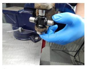
With the spider resting in the bottom yoke, install the bottom bearing cap.
