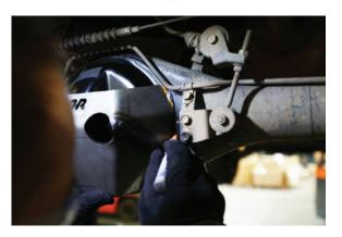
**Tech Tip:** At this point we recommend painting the area of the differential (circled in red) that will be covered by the differential armor.
