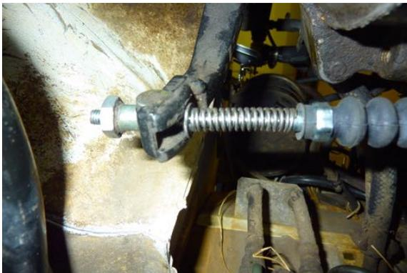
Photograph of Clutch Cable adjustment Nut
