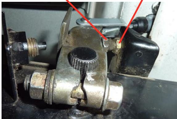
Pedal Lever      Pedal Shaft
