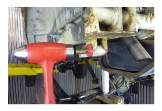
Drive the sleeve in with a hammer.
