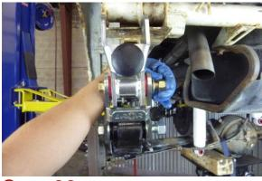
Install the supplied washer and nylock nut, but do not tighten the nut at this point.
