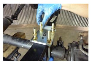
Install the second U-bolt, (2) lock washers and (2) nuts as shown. Tighten these (4) nuts to about 25 ft. lbs. which is 1/2 the specified torque using a 19 mm box end wrench.
