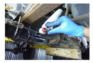
Disconnect the lower shock mount using a 14 mm socket.
