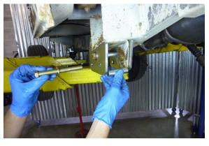
Install the second 1/2X20X4.5" bolt and 2-1/2" sleeve in the holes you just drilled.
