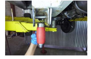
Position the spring mount sleeve and install the supplied 1/2X20X4.5" bolt.
