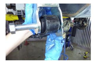
Insert the second supplied spacer washer Size C between the spring and the shackle as shown and insert the bolt the rest of the way through.
