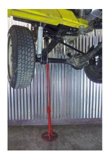
If you are using a twin post lift we recommend using a high lift safety stand (or "Pogo Stick") under the front of the vehicle to make things a bit safer.
