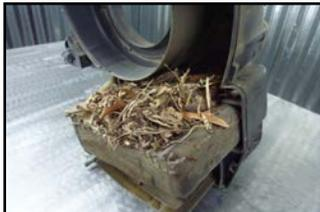
The most common cause of low air flow is leaves and other debris falling down your hood vent into the heater core area. You are probably like
