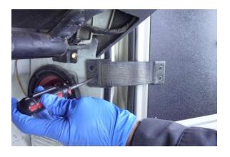
Step 2 Remove the (2) screws from the kick panel side of the door strap using a phillips screwdriver.
