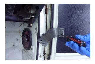
Step 3 Remove the (2) screws from the door side of the door strap using a phillips screwdriver.
