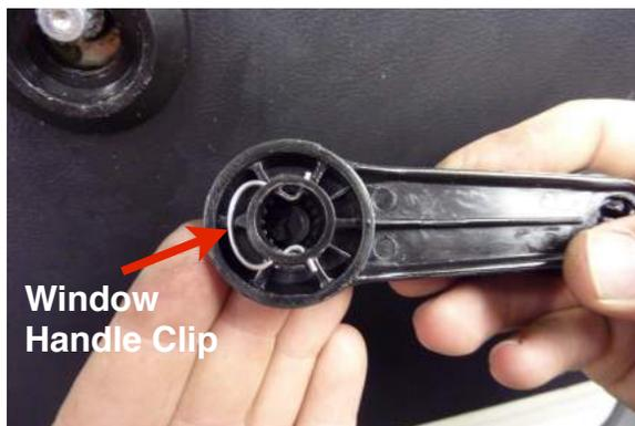
*This picture shows the clip that needs to be removed in order to remove the window handle.*
