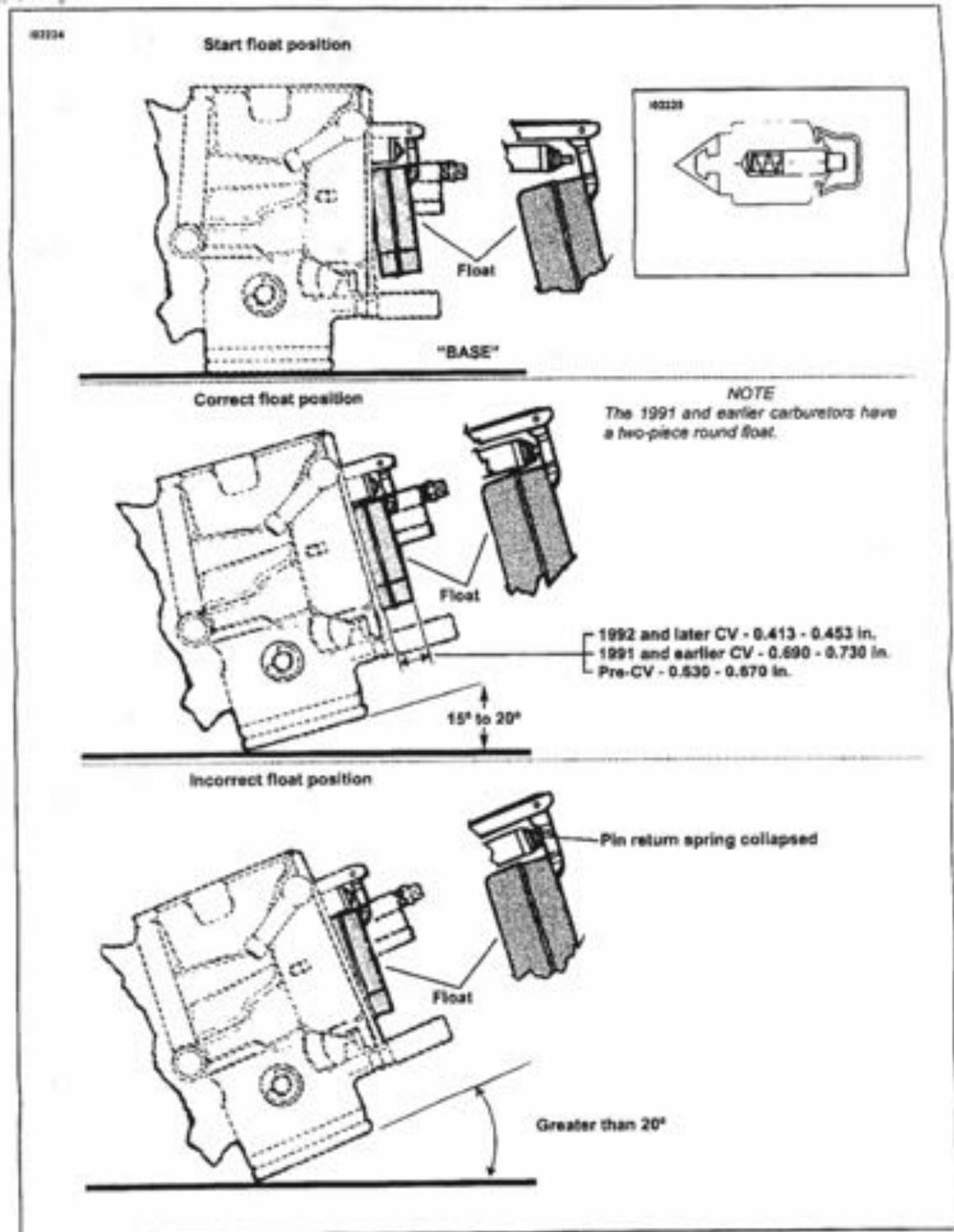
Figure 1. Float adjustment
