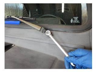
Step 5 Remove the wiper nut using a 10mm box end wrench.
