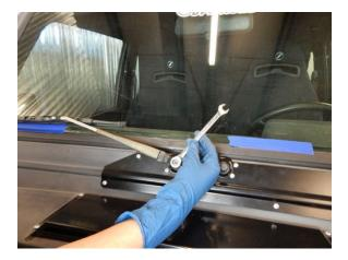
Step 20 Once the wiper arm is positioned correctly, tighten the nut.
