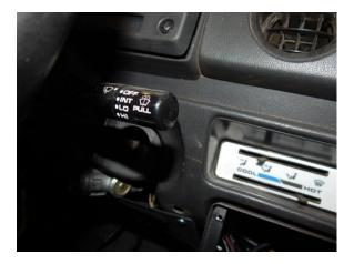
Turn the ignition key to the ON position and turn the wipers to LOW. After several wiper sweeps, turn the wipers OFF. The wipers should now be in the PARK position.
