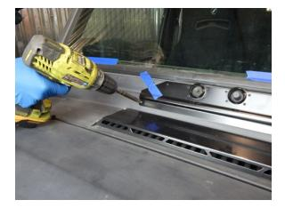
Install the second self drilling screw on the passenger side of the brace and remove the masking tape.
