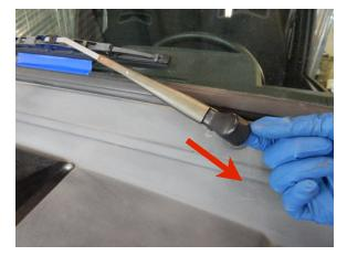
With the cover at about a 45° angle, remove the cover by pulling it toward you.
