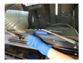
Step 23 Remove the masking tape from both sides of the windshield.
