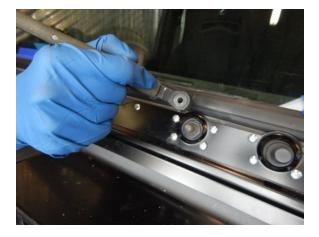
Step 16 Place the passenger side wiper back on the wiper shaft.
