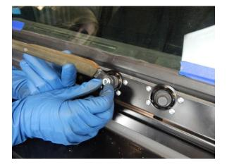
Step 17 Install the nut but leave it loose enough for the wiper arm to be moved easily.
