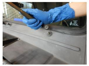
Step 7 Remove the wiper arm from the shaft.
