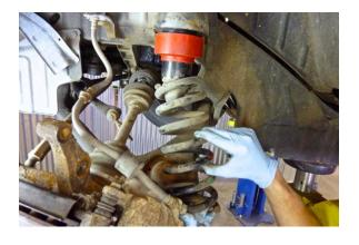
Reinstall the coil spring; top first and then the bottom.
