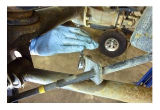
Disconnect the park brake cable bracket using a 10 mm socket or box end wrench.
