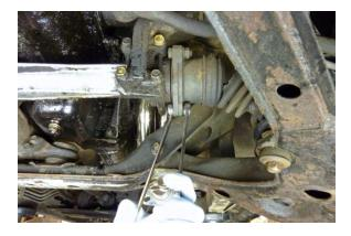
Disconnect the drive axle at the inner end by removing the three bolts using two 14 mm combination wrenches.
