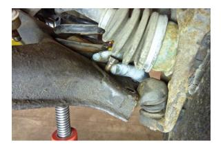
Reconnect the lower ball joint to the lower control arm by installing the (3) bolts.
