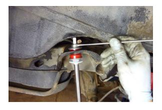
Tighten the nut using a 14 mm combination wrench until the nylon bushings begin to bulge.
