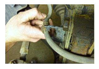
Detach the flexible brake line from the support bracket.
