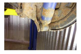
Disconnect the shock absorber by slightly lowering the rear axle assembly.
