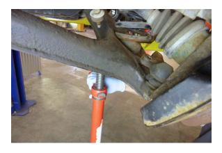
Lower the control arm with the floor jack (or hoist jack stand) which will decompress the coil spring.
