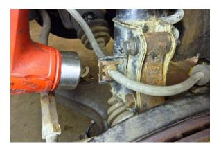
Install the clip by tapping it into place with a hammer.
