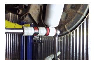
While holding the nut with a 17 mm box end wrench, tighten the bolt using a 17 mm socket until the rubber bushing bulges.
