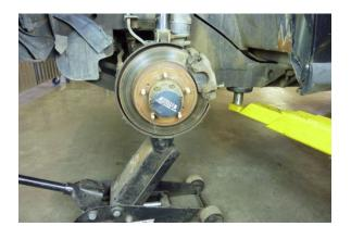
Place a floor jack (or hoist jack stand) under the lower control arm and lift up slightly.
