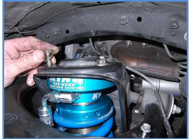
8. Install reservoir in the reservoir bracket using the provided hose clamps. Position the reservoir so it is centered in the cradle with the hose pointing almost straight back. Adjust accordingly.
