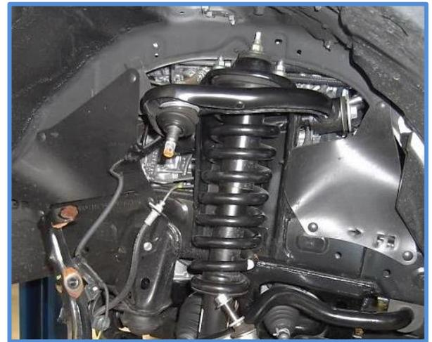
**For Lexus GX470 you will need to remove and unplug the control module on top of the shock.**
