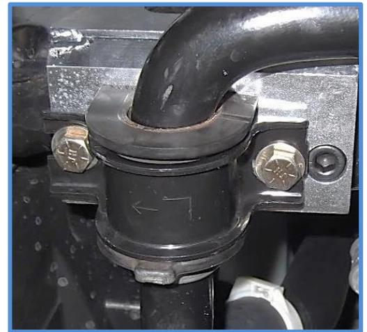
**Some vehicles may require installing spacers to drop down the skid plate supports to make room for the sway bar...**
