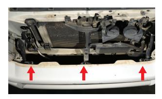
**4.** Remove the clips and screws that retain the bottom center part of the bumper to the factory crash bar.
