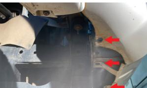
**6.** Disconnect both fog lights. Then remove the front bumper starting on one side and going towards the other side. Use caution when pulling the sides of the front bumper away from the vehicle. If necessary, use a small pick to disengage the plastic clips that secure the top of the bumper to the sides of the body.
