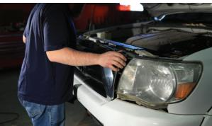
**11.** Install the new bumper using the original crash bar mounting nuts. The bumper can be adjusted vertically to achieve the necessary clearance between the upper edge of the new bumper and the original plastic bumper.
