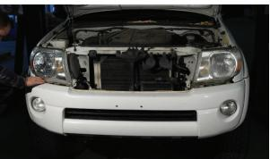
**7.** Remove the factory crash bar. It may be necessary to use a mallet to tap the crash bar off the mounting studs.
