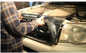
**2.** Remove the (2) clips that retain the trim pieces under the headlights. Remove both trim pieces by prying outwards and then pulling in towards the center of the vehicle.
