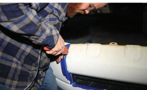
**9.** Using a sharp razor blade, cutoff wheel or body saw, carefully cut the center section of the bumper out along the cut lines laid out in the previous step. If there are any sharp edges or burrs left from the cutting, smooth those out with a file. Remove the masking tape.
