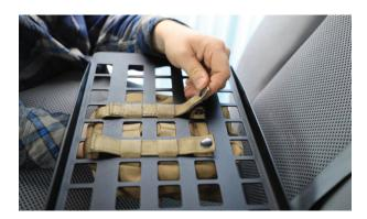
**3.** Position the rack on the interior of the roof and align the mounting slots in the rack with the mounting holes in the roof. Use the original grab handle mounting bolts to bolt the rack to the roof. If desired, place the original grab handles or after-market grab handles over the mounting holes in the rack and reinstall the mounting bolts.
