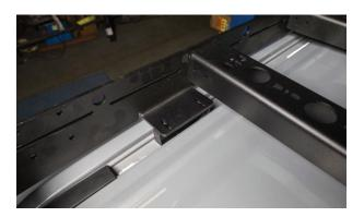
**13.** Using the supplied hardware, bolt the roof rack to the roof of the vehicle. Apply a small amount of sealant on the threads of the bolts to ensure the joints are leak proof.
