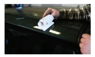
**10.** Apply a generous amount of sealant around the factory mounting locations as shown using the supplied sealant. Align the holes in the supplied mounting blocks with the holes in the roof and set the mounting blocks on top of the roof. The mounting block with the holes closer together is for the forward mounting location. Apply light pressure to seat the mounting blocks against the roof.
