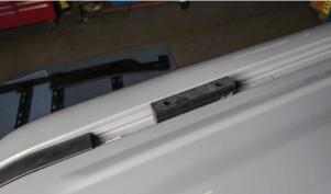
**11.** With the mounting blocks in place on the roof, if desired, trim the factory weather stripping so it sits in between the mounting blocks on the roof. It is helpful to lay the weather stripping on the roof by the mounting blocks and then mark the cut locations. Once the weather stripping is trimmed, use the provided VHB tape as needed on the underside of the weather stripping to secure it in the roof channels.
