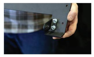
**8.** Apply the provided trim to the bottom edge of the front deflector as shown. Mount the front deflector to the front mounting brackets using the provided ¼" bolts, flat washers, and lock nuts. Initially position the deflector so the top bend is even with the top of the side rails. Hand tighten the deflector mounting bolts so the deflector can be easily adjusted later.
