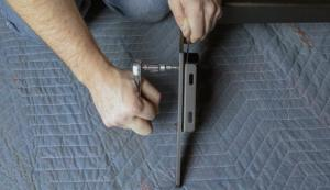
**7.** If you plan on mounting a light bar to your front deflector, mount the light bar brackets to the front deflector with the provided hardware as shown. Mount the desired light bar between the mounting brackets.
