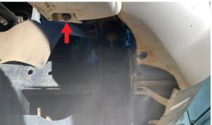
**6.** Disconnect both fog lights. Then remove the front bumper starting on one side and going towards the other side. Use caution when pulling the sides of the front bumper away from the vehicle. If necessary, use a small pick to disengage the plastic clips that secure the top of the bumper to the sides of the body
