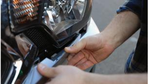
**3.** Remove the (3) clips that retain the top center part of the bumper to the vehicle.
