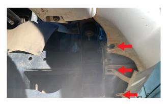
**5.** Remove the (2) screws that retain the inner fender liner to the bumper. One screw is located at the bottom of the bumper and the top screw is accessed through a hole in the fender liner as shown. Remove the plastic clip between the (2) screws by rotating 90 degrees and then removing. Repeat the process on the other side of the bumper.
