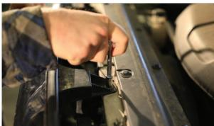
**2.** Remove both trim pieces under the headlights by prying outwards and then pulling in towards the center of the vehicle
