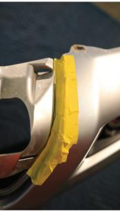
**10.** Using a sharp razor blade, cutoff wheel or body saw, carefully cut the center section of the bumper out along the cut lines laid out in the previous step. If there are any sharp edges or burrs left from the cutting, smooth those out with a file. Remove the masking tape.
