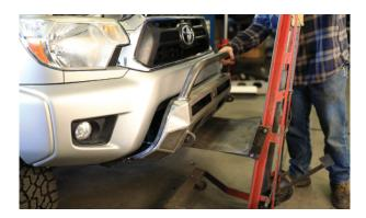
**14.** Install the provided side support brackets and supplied hardware to connect the lower corners of the factory bumper to the new bumper. The brackets can be swung forward or rearward so the gap between the original plastic bumper and the new bumper is minimized.
