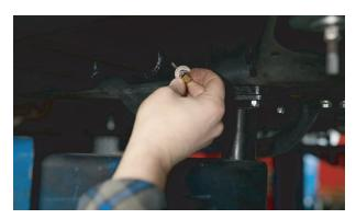
**5.** Once the rock slider is supported on the frame rail, reinstall any brackets you may have previously taken off on top of the slider mounting bracket. On the driver's side the front mounting plate will go under the KDSS lines. Snug a few of the mounting bolts so the rock slider is pulled against the frame rail but you can still adjust the position of the slider.
