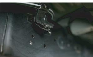
**3.** If your vehicle is equipped with the KDSS, remove the brackets holding the KDSS lines to the frame and small skid plate protecting the KDSS lines going under the frame.
