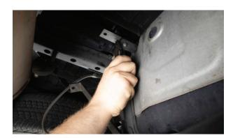
**12.** Tighten all installed bolts. DO NOT exceed 33 ft-lbs when tightening the front bolts going into the nut plates.
