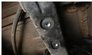
**3.** Assemble the front skid piece to the main skid piece using the supplied 3/8" carriage bolts, washers, and lock nuts.
