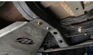
**5.** Install the rear driver and passenger skid mounts onto the skid plate as shown using the supplied hardware. The passenger mount is the longer mount and the driver mount is the short mount. Do not fully tighten these bolts yet.
