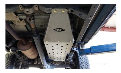
**1.** If equipped, remove the factory fuel tank skid plate by loosening and removing the (4) mounting nuts.
