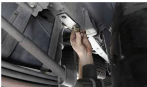
**9.** Using the supplied hardware, attach the secondary mounting bracket to the factory cross member as shown. About half of the bracket should be supported by the factory cross member and the other half should hang off. Align the bracket so it is in line with the cross member and tighten the mounting bolt.
