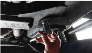
3. Install the rear 3 bolts with the rectangular nut plates finger tight.
