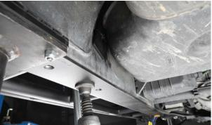
**9.** In the inside of the frame near the middle of the slider; there are two plastic clips that hold brake lines that will need to be removed. Insert the welded nut plate into the hole with the nut on the inside of the frame as shown. You may need to use a screwdriver to move the brake lines in order to install the plate. Fasten with the M12-1.75x95 bolt with flat and lock washer.
