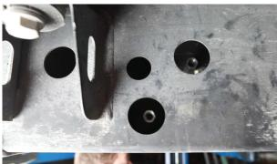
**5.** Remove the 2 bolts from frame toward the front of the frame as shown. You will have to pull the wiring harnesses clips off the frame in order to get access to the top bolt.
