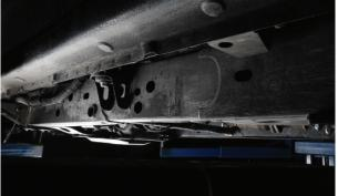
**3.** Using a 13mm socket and an extension remove the two nuts in the larger frame holes.
