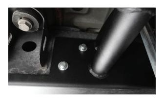
**11.** When installing the M8 bolts you will use a lock washer and the wedge washer. When installed correctly the thick side of the wedge washer will be on the right side as shown.
