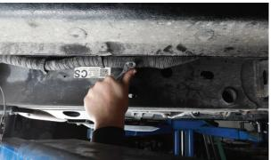
6. Install the square nut plate into slot on crossbar and center as shown.
