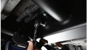
**12.** Be sure the slider's bottom edge is flush with the frame. Then tighten all bolts.
