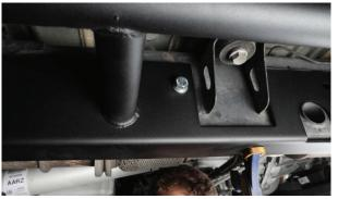
**4.** Install the 2 long M12 Bolts with the double nut plate. The flanged ends will be touching the frame with the short flange toward the front of the vehicle.
