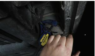
**2.** Using a 10mm wrench, remove the nut holding the e-brake assembly together. Save the nut and bracket for re-installation. Move the brake lines out of the way to allow for slider installation.
