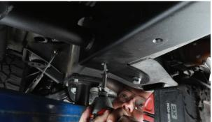
**15.** Feed the E-brake lines through the gussets as shown. Re-install the bracket and tighten the nut down until you reach the amount of exposed thread that was there prior to install.
