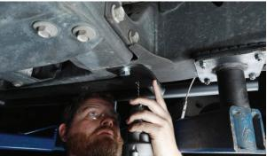
**14.** Install the self-drilling flat head screws with a drill and a Phillips #2 bit until it's flush with the surface.
