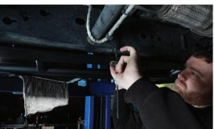
**8.** Using the welded nut plate as shown, insert the nut side of the plate to the frame hole so it will be facing away from the fuel tank. Fasten with the M12-1.75x95 bolt with flat and lock washer.
