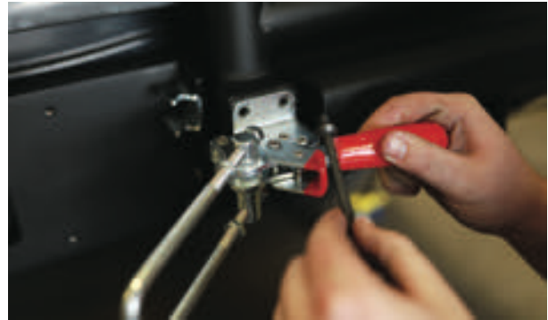
Hold the assembled latch up to the swing arm and begin to add the provided bolts as shown. Once properly aligned, torque all four bolts to 18ft-lbs.
