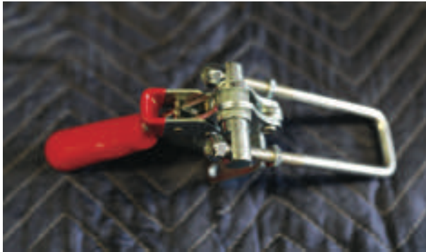
Thread the nylock nuts provided as far as you can by hand for now.
