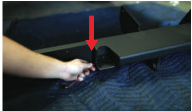
Feed the wires through the hole on each side of the license plate area.
