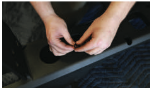
Feed the wire through the nut and proceed to tighten the nut down on the LED light.
