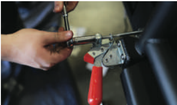
Hook the U-bolt to the anchor bracket and close the latch. From here begin to tighten the nylock nuts to set the clamping strength for the swing arms. They should take some force to close but you shouldn't have to muscle it. You may have to test and adjust the nuts a few times to get the desired feel. Once that is complete tighten the jam nuts up against the swivel bar. Repeat this process for the other swing arm.
