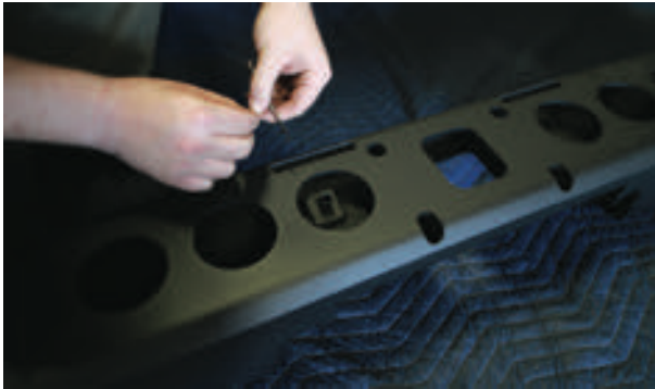
Flip the bumper over and use a small screwdriver as shown to install the small mounting screws.
