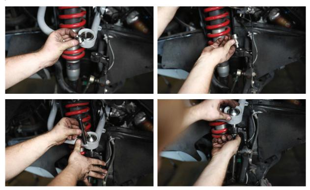
**8.** Use a zip tie to secure the ABS wire to the tab on the rear of the UCA and apply the All-Pro decal to the outer side of the UCA. Secure the inner fender covers using the existing plastic snaps.
