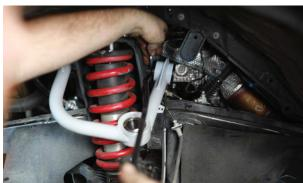
**6.** Once the pivot bolt is all the way through the UCA, put a new washer and the stock nut back on the pivot bolt and snug the nut. Before fully tightening the nut, grease the UCA bushings using a grease gun on the zerks already installed on the UCA until grease comes out between the bushings and the washers. Once the bushings are greased torque the pivot nut to 85 ft-lbs. Wipe any excess grease off the UCA.
