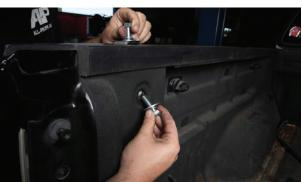
**3.** Remove the bolt that was used to help position he bracket. Make sure the top of the bracket is not protruding above the bed sides. Repeat steps 2-3 on the rest of the stake pockets.
