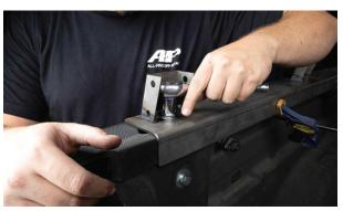
**6.** Using the hardware shown begin installing the vertical brackets on the saddles closest to the cab on both the driver and passenger sides. The install the button head screws and corresponding hardware as shown below. Leave them finger tight for now.
