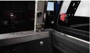
**7.** Install the connector brackets in the orientation shown above. Use the same set of hardware to attach the vertical brackets and leave them finger tight for now. Do this on both sides.
