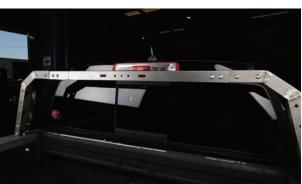
**9.** Use a long straight piece of material and clamp it to the top of the crossbeam assembly to align all of the parts together. Then tighten all hardware of this assembly. Repeat steps 6 through 9 for the next two crossbeam assemblies.
