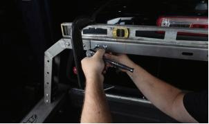
**10.** Using the hex head screws, corresponding lock and flat washers, and hex nuts. Install the boxed cross bar in the center of the main crossbeam assemblies as shown. Tighten down the hardware at this time. Repeat this between the next set of crossbeams.
