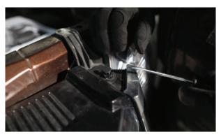
**4.** Remove bolts holding the fog light frame to gain access to the remove the parking sensor and fog light wiring. Un-clip the wiring harness from the fog light frame.
