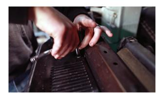
**3.** Pull bottom portion of the grille off. There will be resistance but the lower clips are designed to pop off. When pulling grille off of the vehicle make sure all wiring is disconnected as some models may have different wiring/sensors mounted in the grille.
