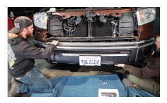
**8.** Remove any necessary wiring still attached to bumper.
