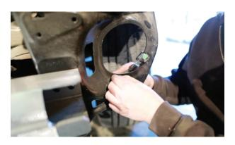
**10.** Remove 8 bolts holding crash bar onto vehicle. Save the hardware as it will be reused to install the Apex bumper.
