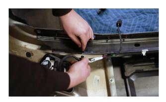
**9.** Remove wiring clip as shown.
