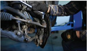
**8.** Remove the sway bar nut and remove the sway bar from the spindle..
