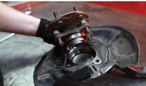
13. Remove the ABS sensor from the knuckle.
