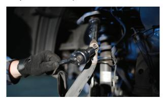
**9.** Remove the upper ball joint and tire rod from the knuckle.
