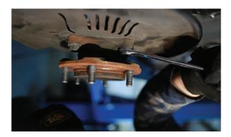
6. Remove the cotter pin from the upper ball joint and loosen the upper ball joint nut.
