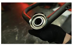
**6.** Install the snap ring into the snap ring groove in the uniball cup. Make sure that the snap ring is fully seated in the snap ring groove.
