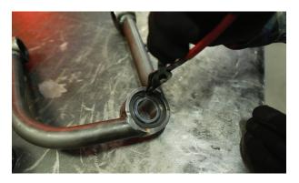
2. Take the small tool and place it on the top side of the uniball (side without a snap ring). Be sure to center the tool on the uniball. Take the large tool and place it on the snap ring side of the uniball cup. Be sure to center the tool on the uniball cup.
