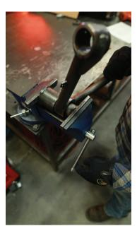
**4.** When pressing the uniball out of the uniball cup be sure not to drop the uniball or the control arm.
