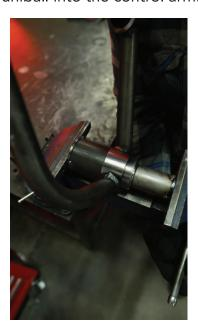
**4.** Once the uniball is started into the uniball cup it may be necessary to remove the control arm from the pressing tool if the uniball is pressing into the uniball cup at an angle. If so, place the small tool on top of the uniball and use a soft-face hammer to straighten the uniball in the uniball cup.
