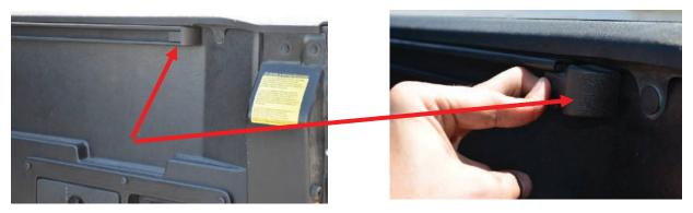
3.) Insert bed rail mounting bracket into stock bedrail slides. Two brackets are used for each side (passenger and driver). Positon brackets so that one is near the ca and one is near the tailgate side of the stock bed rail tracks.
