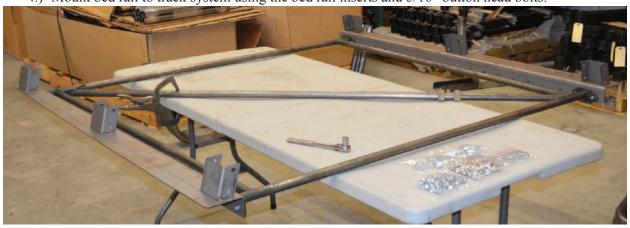
5.) Mount vertical bars into the bed rail saddles using 4 3/8" button heads, 4 flat washers, 4 lock washers, and 4 nuts. Make sure to leave everything loose throughout assembly, tighten only once everything is fitted properly.
