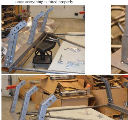
6.) Place horizontal cross bars on top of vertical bars and bolt them using 8 3/8" Button heads per cross bar.
