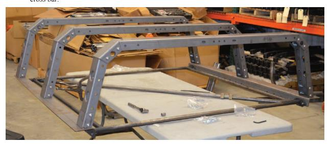
7.) Next, mount accessory cross bars using the 3/8" hex head bolts. AllPro recommends two accessory crossbars between the two rear hoops, and two down the middle in between the horizontal cross bars.
