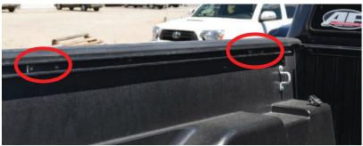
4.) Mount bed rail to track system using the bed rail inserts and 5/16" button head bolts.
