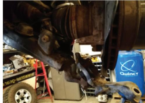
**6.** Unbolt and remove the lower A-arms from the frame.
