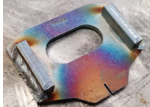
**12.** Flip the bracket over and plug weld the tabs to the bracket.
