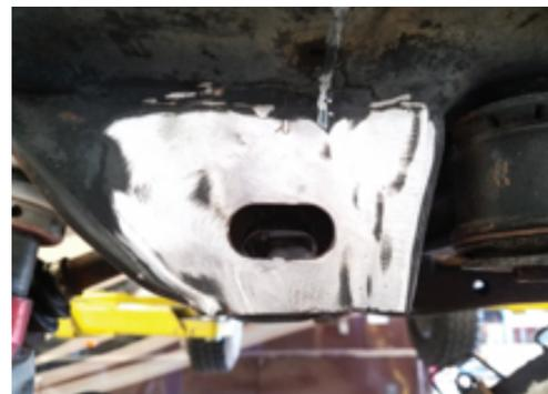
**10.** Install the tabs into the LCA gussets. You may have to gently tap them into the bracket with a hammer.
