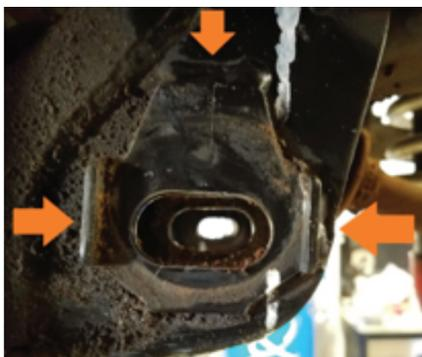
**9.** Using an angle grinder, grind the surface of the frame down to bare metal. The surface should be flat and free of paint.
