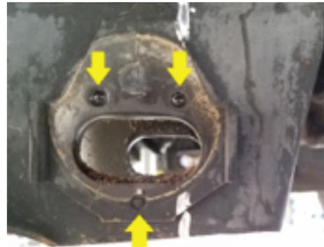
**8.** Using a cutting wheel, cut the welds on the rear stock alignment cam tabs. Using a chisel, carefully remove the stock alignment cam tabs from the frame. Repeat for the (3) remaining rear stock alignment cam tabs.
