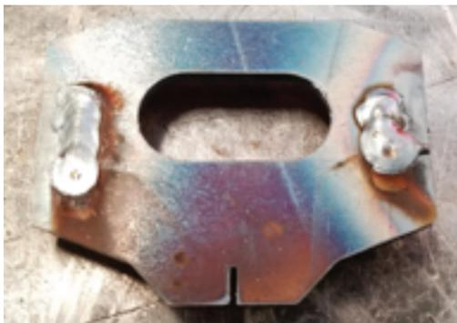
**13.** Grind the welds on the backside flush with the gusset using an angle grinder. Repeat Steps 10-12 for the remaining gussets.
