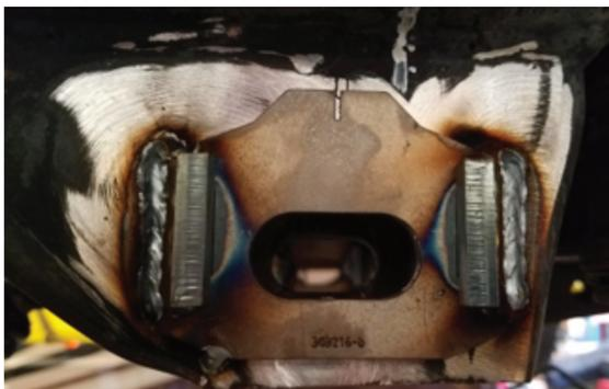
**15.** Make sure the cam bolts and cams rotate freely in the slots and between the gusset tabs.
