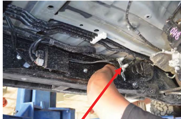
Bracket and lines moved in order to allow installers arm to fit into frame cutout
