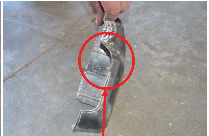
Cut out on top of plastic cover must be trimmed opened more on right side.
