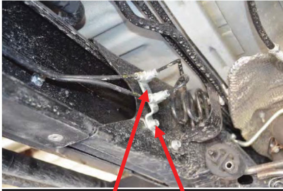
Brake Line Bracket Bolt to remove
