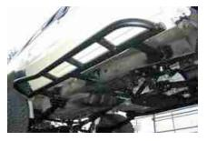
small amount of material on the pinch weld of the body directly above each of the three support bars. When mounting Rock Guards there should be a 1/4" gap between the bar and body. This prevents noise and vibration from being transmitted from the frame through to the body.
