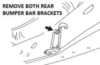
2. Begin removal of the rear bumper cover taking care not to break any mounting tabs of the plastic corner panels. Remove the rear bumper energy absorber, side stays, side support sub-assemblies, rear bumper bar brackets and the tow point.
