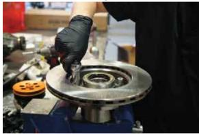
**STEP 18** Grease inner wheel bearing and set into race.
