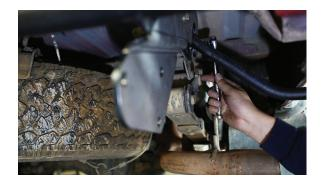
**9.** Tighten the bolts to the hitch
