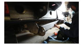
**7.** The order for the hardware bolt, washer, part/frame, washer, split lock washer, nut (hitch screws)
