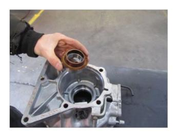
**STEP 12**Re-attach the rear transmission housing with 7 bolts and install sleeve
