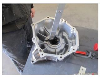
**STEP 10**Support bearing removed.
