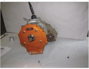
**STEP 4**Install provided coupler to the transmission.
