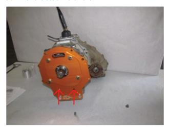
**STEP 14**Install the seal housing with a rubber mallet.
