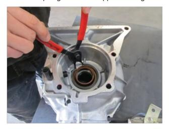
**STEP 9**Remove the rear support bearing.
