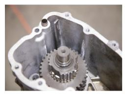
**STEP 31**Area to clearance for counter shaft gear.
