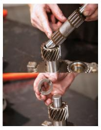
**STEP 35**Install 4WD shift fork and collar over hub.
