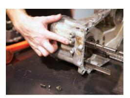
Insert the bushing locking ball into shaft, secure using a
