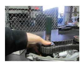
**STEP 40**Support main shaft and press bearing onto shaft and install C-clip.
